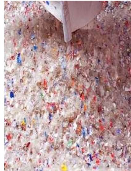
Shredded plastic used for Asphalt road construction.
